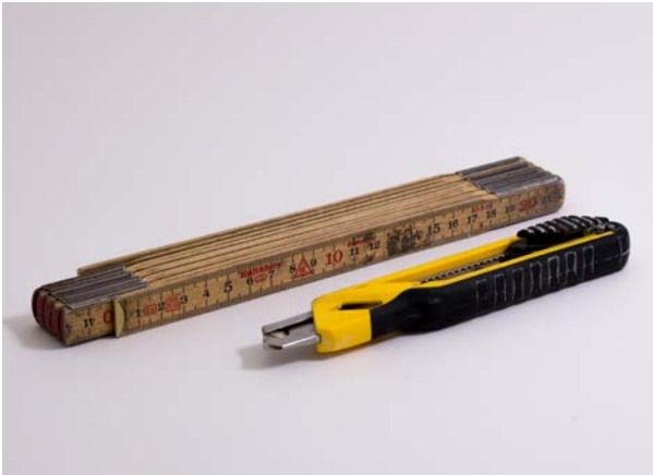
1. Knife & measurement tool To measure and cut the acoustic boards
