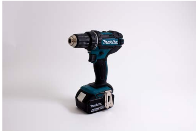
2. Screw gun To fix the acoustic boards mechanically
